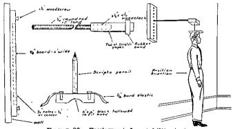
FIGURE 36.- Equipment for stability test.
